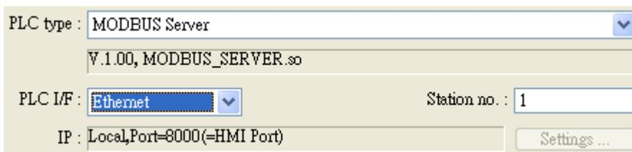
For MODBUS Server and HMI use the same port no., please change the MODBUS Server port no. on Model tab of System Parameter Settings.
