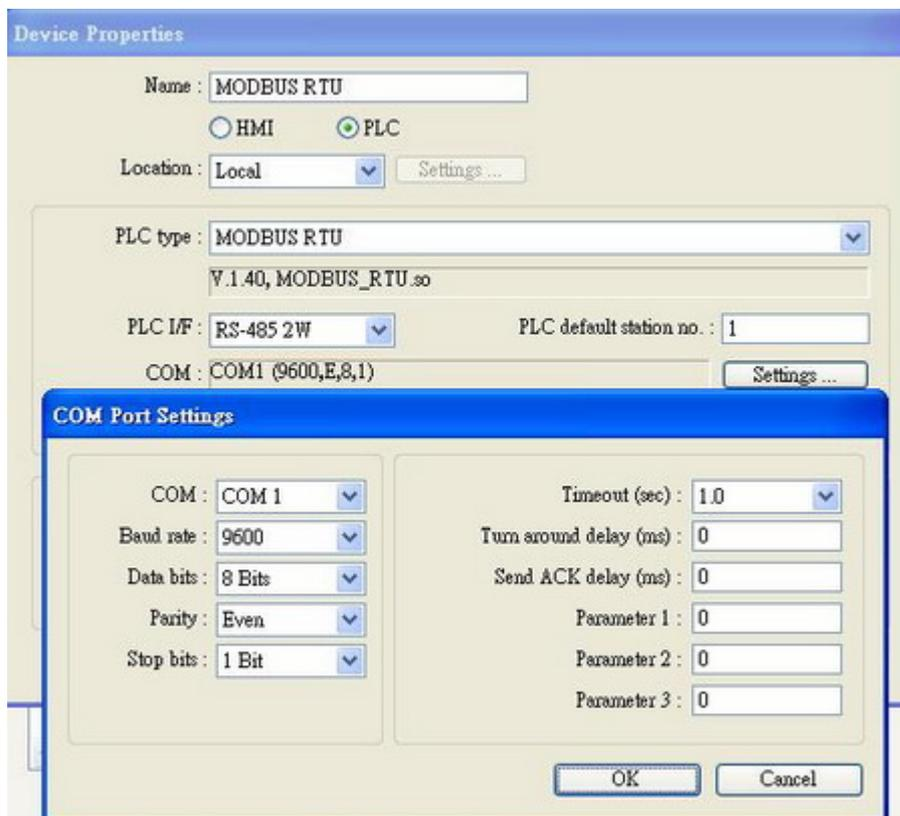
Set and click OK, a new device "MODBUS RTU" shall be listed in the Device tab.
