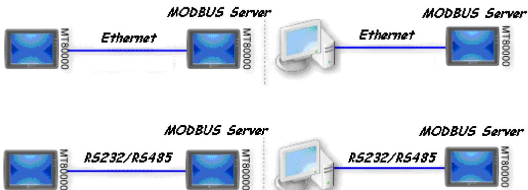
Refer to the above illustration, it shows MT8000 is set as MODBUS Server. The HMI, PC or other devices can use MODBUS protocol to read or write the data from MT8000 via Ethernet or RS232/485 interface. Please follow the steps as below.
