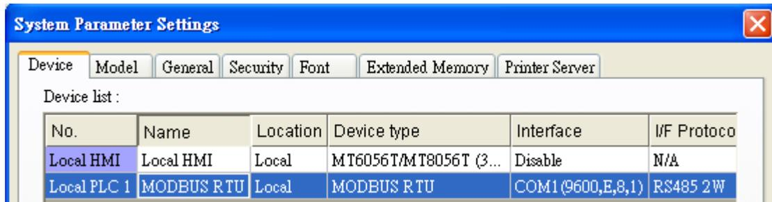
In the setting page of each object, there is an "MODBUS RTU" in the PLC name selection list, you can then select appropriate device type and address.
