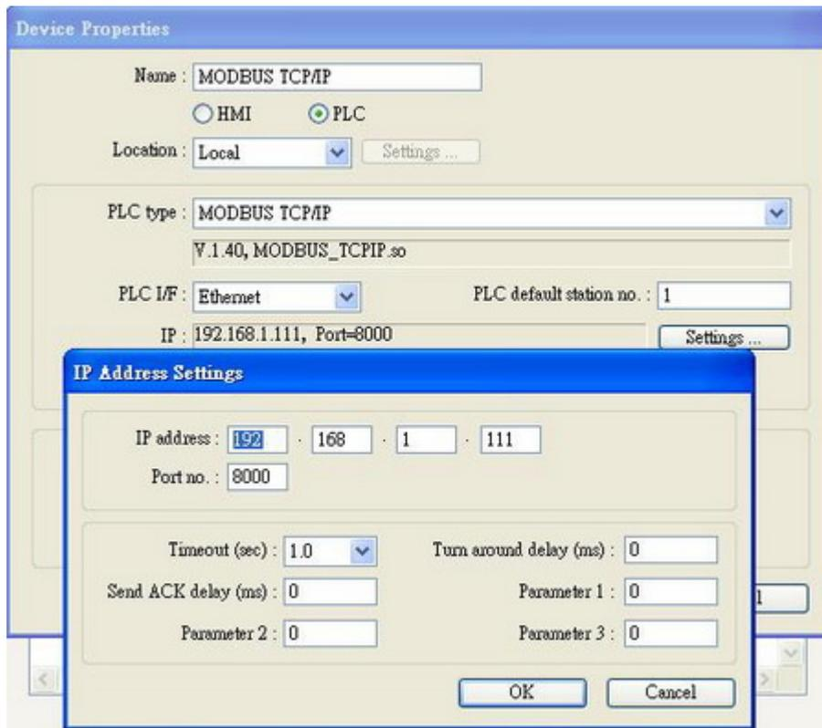
If the client use RS232/485 interface, the PLC type must be set as "MODBUS RTU", please make sure the communication parameter setting is correct.
