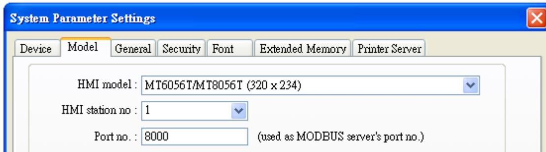
After finishing the setting, MODBUS Server will be list on Device tab.
